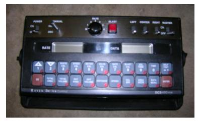
rates to be programmed for different road conditions. This system also gives a blast option which will allow the drive to add extra product in severe conditions.
