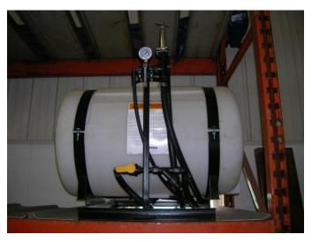
The ATV units are a skid sprayer that will fit into the bed of most ATV type machines. They come with a 55 gallon tank, regulating valve, return line and your choice of either a gas or 12 volt electric pump. The 12 volt electric pump unit is pictured. This unit also comes with a hand wand and 20' of hose for spraying hard to reach areas. On the back of the sprayer is your choice of a 12' or 7' boom. Like the 3pt unit this boom is capable of having spray
