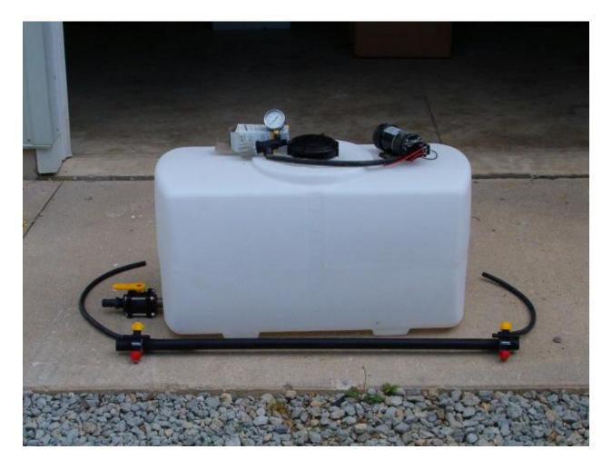
This pre-wet unit is designed to slide beside a salt applicator in the bed of a smaller truck. This unit will apply a small amount of product to the salt to help it react quicker with the ice and snow. The tank is a Snyder PCO tank and comes in multiple sizes to fit your particular needs. This unit comes with a john-blue 12 volt electric pump and a rheostat in the cab to adjust the flow of the product. It comes with a quick fill to make refilling the tank a quick process.
