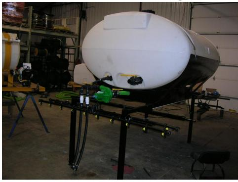
The 1000 and 2000 gallon deice units are made to slide into a dump truck or similar size vehicle. As you can see in the picture these units come with a stand that folds and unfolds as the unit is slid in and out of the truck. This particular unit has a hydraulic
