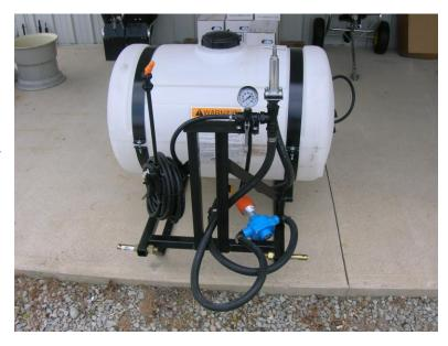
application of different areas. There is a manual shutoff for the boom and a manual pressure adjustment to get the correct amount of product on.
