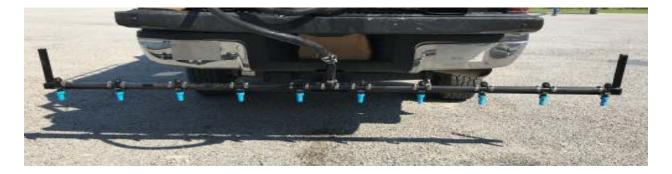
To make sure the deice product gets to the road surface to be treated correctly, we offer several different boom options. The picture above shows a standard 96" boom with either nozzles or drops. The nozzles work better in areas with less traffic because it accomplishes complete coverage of the area, such as driveways and parking lots. The drops work better in areas of high traffic, since the traffic
