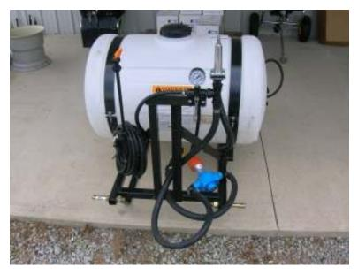
nozzles or dribble hose for application of different areas. There is a manual shutoff for the boom and a manual pressure adjustment to get the correct amount of product applied.
