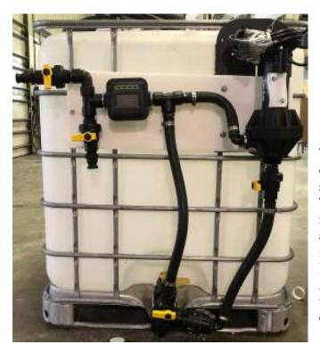
This system easily mounts to an existing tank with frame or another style tank with appropriate framework. The 12 volt Dura-Pump provides the required flow volume for deice and anti-ice liquid applications. This pump is capable of handling high viscosity liquids in low temperature conditions. All the items listed below come with this system to make liquid application easy and effective on small properties:
