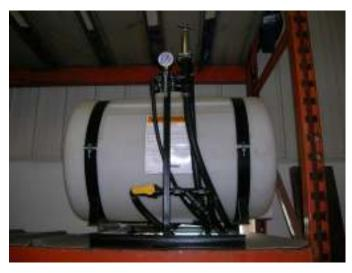
The ATV unit is a skid sprayer that will fit into the bed of most ATV type machines. They come with a 55 gallon tank, regulating valve, return line and your choice of a gas engine driven pump or 12 volt electric pump. The 12 volt electric pump unit is pictured. This unit also comes with a hand wand and 20' of hose for spraying hard to reach areas. On the back of the sprayer is your choice of a 12' or 7' boom. This boom is capable of having
