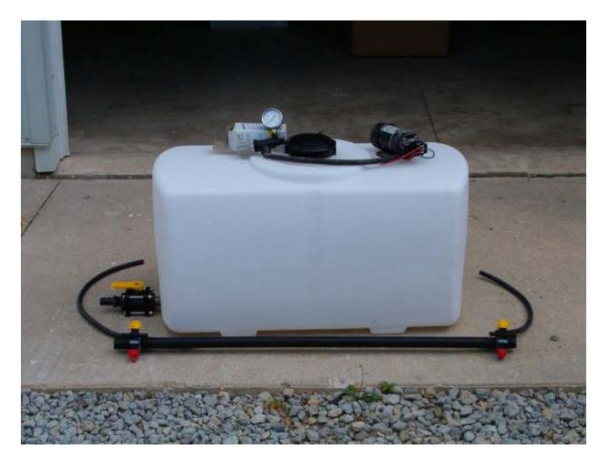
This pre-wet unit is designed to slide beside a salt applicator in the bed of a smaller truck. This unit will apply a small amount of product to the salt to help it react quicker with the ice and snow. The tank is a Norwesco PCO tank and comes in multiple sizes to fit your particular needs. This unit comes with a John-Blue 12 volt electric pump and a rheostat in the cab to adjust the flow of the product. It comes with a quick fill to make refilling the tank an easy process.
