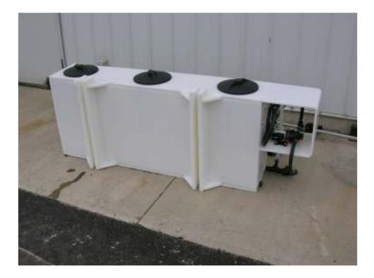
This unit attaches to the tailgate of a salt truck and allows liquid deicer to be applied to the salt as it hits the spinner. By doing this, the salt reacts quicker with the ice and snow to speed up the melting process. This unit comes with a John-Blue 12 volt electric pump and a rheostat in the cab to adjust the flow of the product. These tanks are custom built out of 1" poly to withstand the abuse that they take from being attached to the back of a salt truck.
