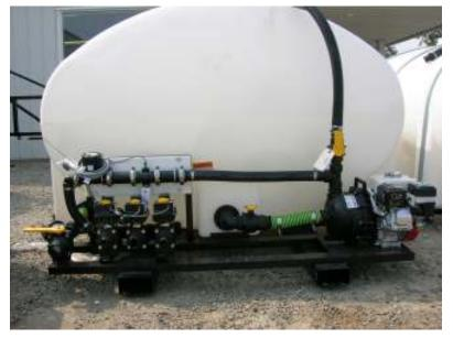
The 1035 and 2000 gallon deice units are made to slide into a dump truck or similar size vehicle. The unit pictured is set-up with a Roadmaster automatic rate controller with plumbing for 3 sections. Also included is a 96" or 80" boom to apply liquid deice product to the road surface. The boom can be equipped with either drops or nozzles depending on the surface to be covered.
